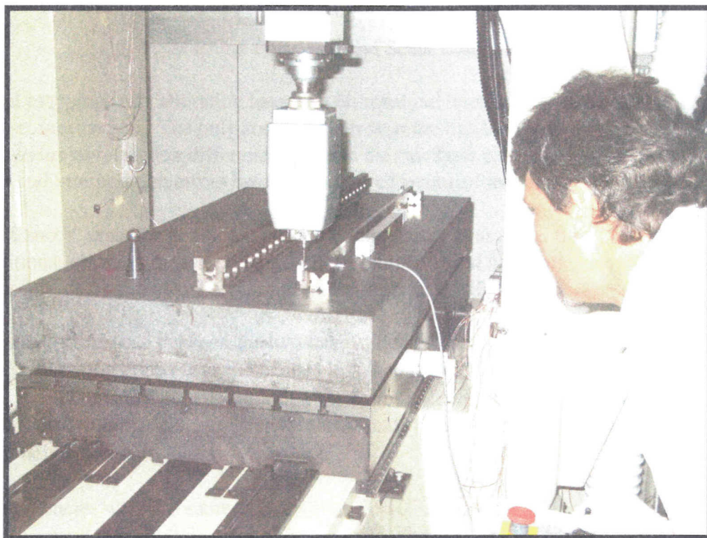
Measurement of the NIST Committee Meter using the M48 Coordinate Measuring Machine
