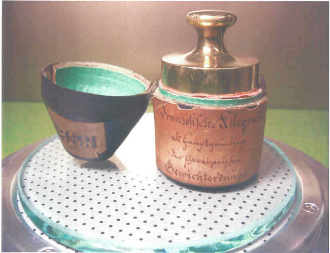
Picture 2: Committee Kilogram within its original protection case
