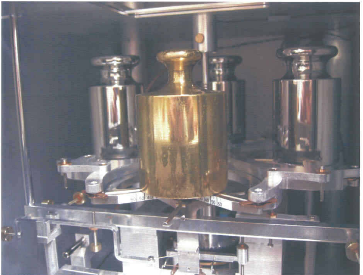
Picture 1: Committee Kilogram inside the primary Mass Comparator of Metas
